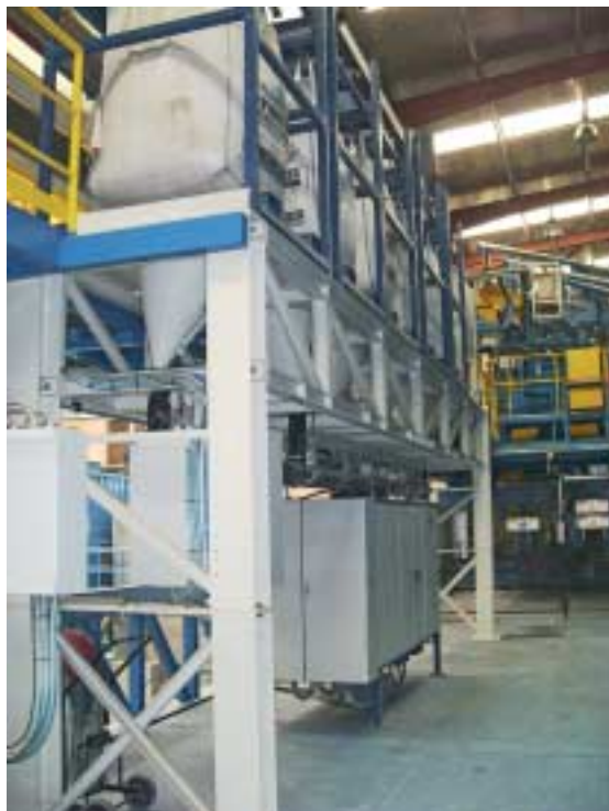
Fig. 1 Six color granule system with three pressure conveying vessels for three mixers.
