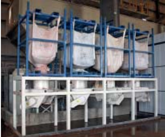
Fig. 4 Four color dry to wet powder pigment system with four Big-Bags.
