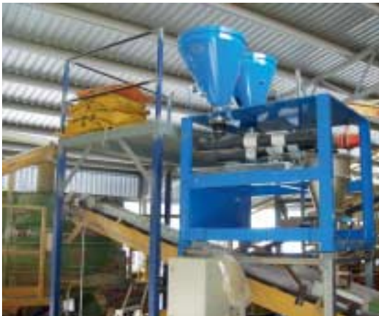
Fig. 5 Two color Würschum system CSR for filling with paper bags.
