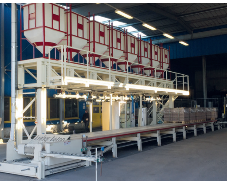
Overview of the system with 8 colour positions in a row
