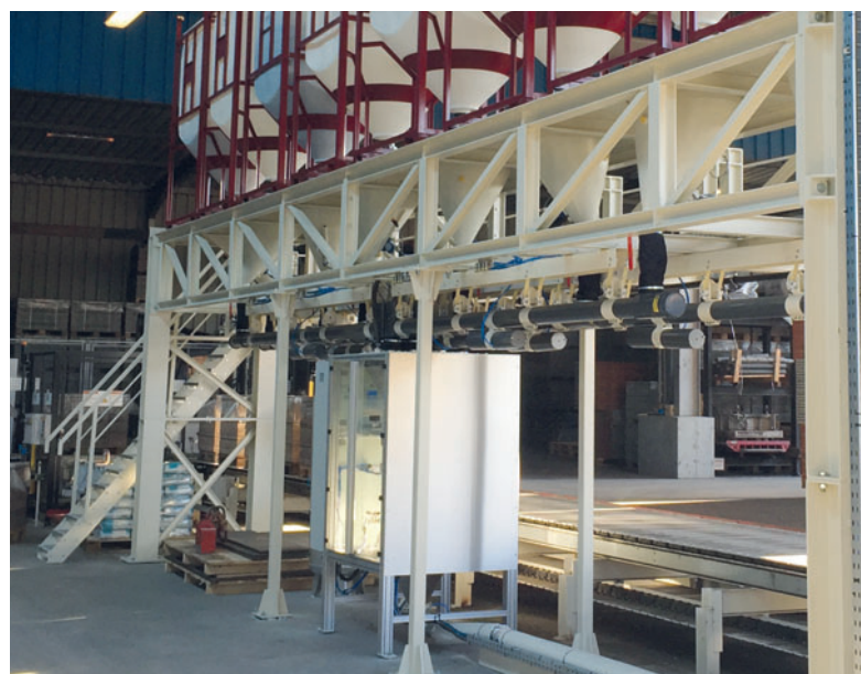
COM 70-1 vibration feeders and precision weighing hopper
