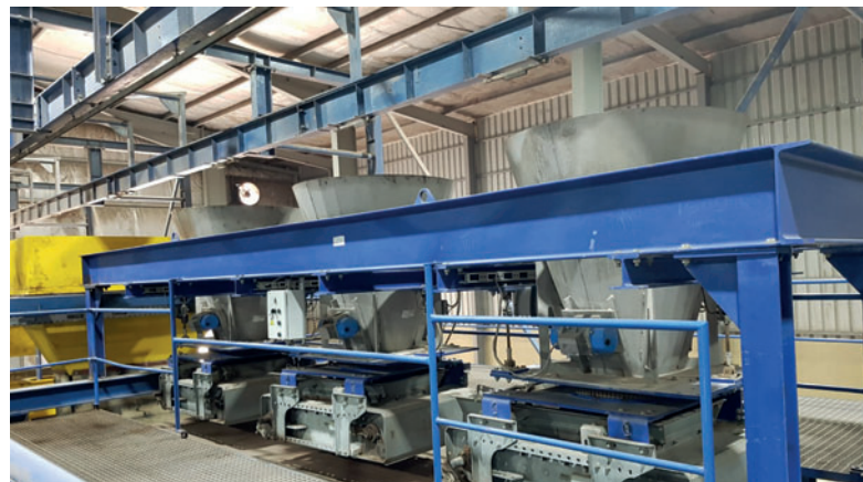
Multi-colour concrete hoppers for face mix
