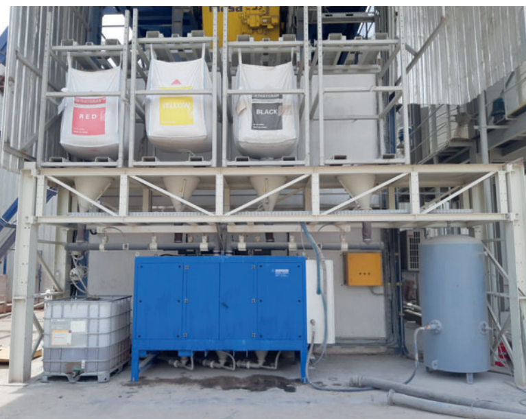
Com 70-3 - granule dosing system with 3 sending vessels
